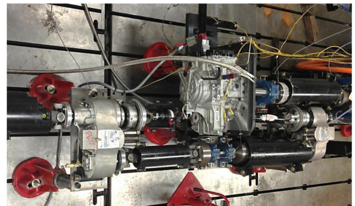
Figure 5. GM6T40 Transmission during testing
