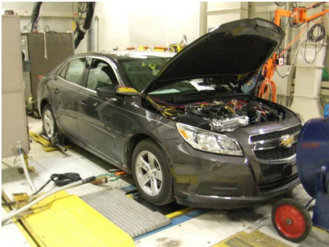
Figure 1. Chevy Malibu undergoing dynamometer testing
