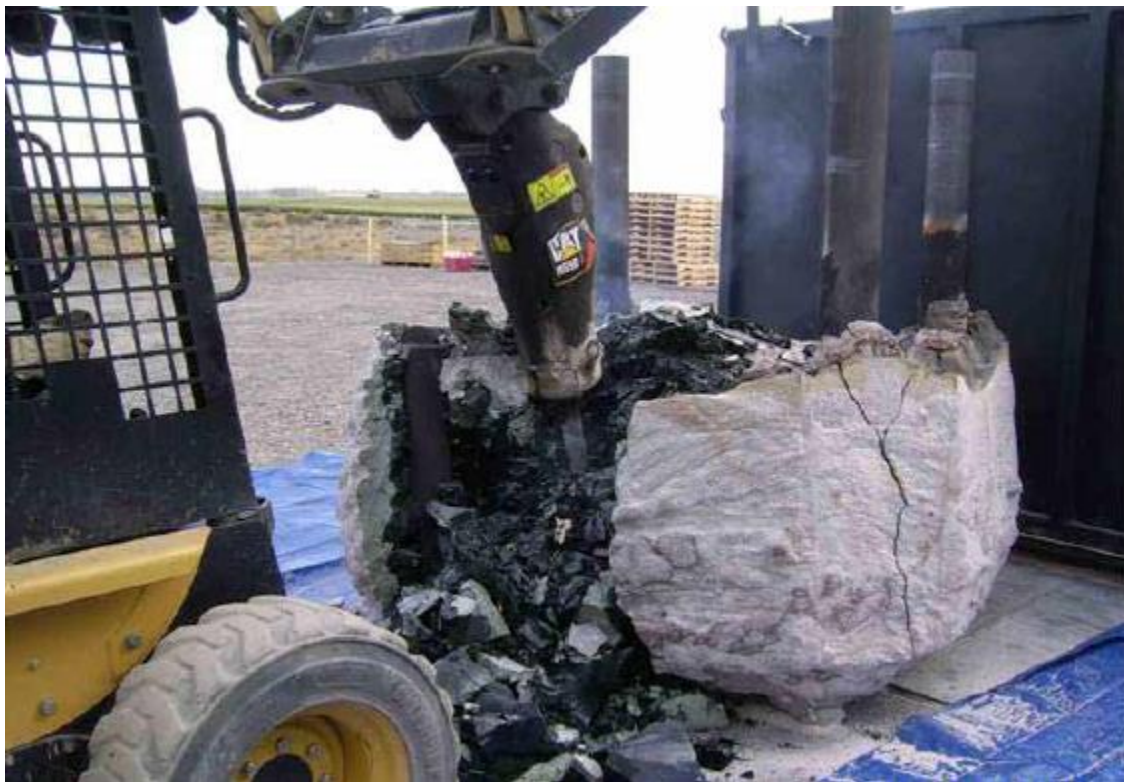
Figure 3: Demolition of Final Glass-like Product to Allow for Sampling During EPA Demonstration
