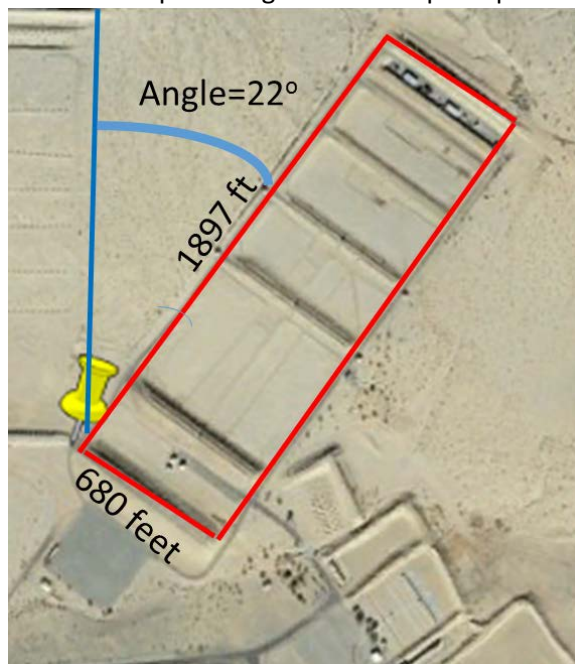
Figure 4-1: Example of Fugitive release point parameters
