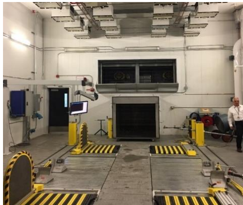
The NVFEL hot test cell chassis dynamometer, with heat lamps on the ceiling simulating vehicle operation in hot environments. (EPA OIG photo)
