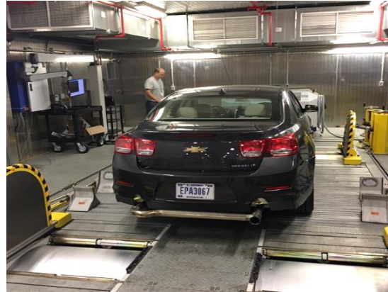
Chassis dynamometer in the NVFEL cold test cell, which simulates driving conditions in below-freezing temperatures. (EPA OIG photo)
