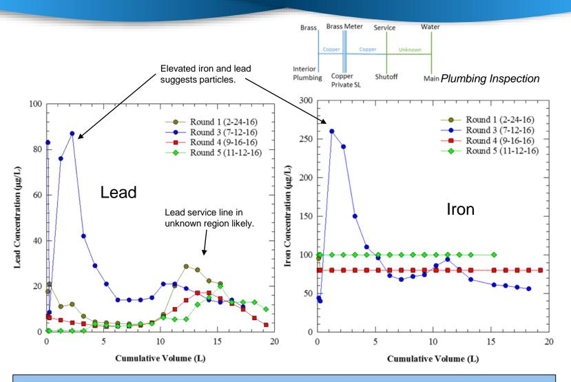
Two lead sources: 1) Associated with iron corrosion – likely particulate lead, 2) From the lead service line – likely dissolved lead.
