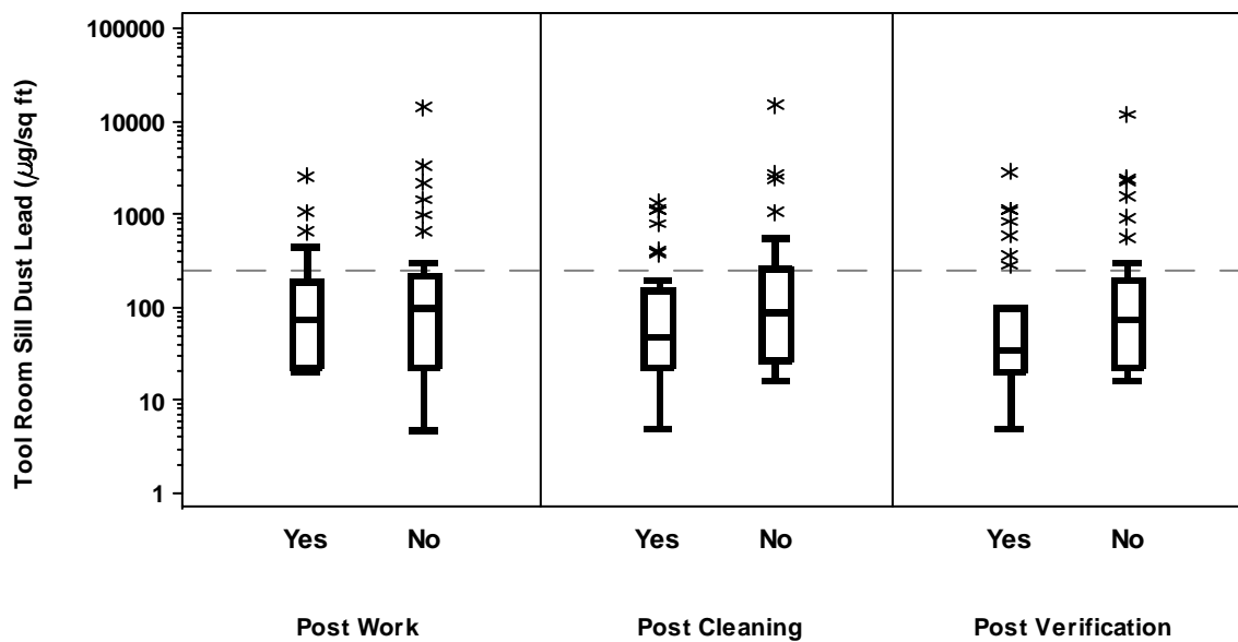
Figure D2.6b. Box Plots of Sill Dust Lead Loading in the Tool Room by Stage and Rule Plastic Use
