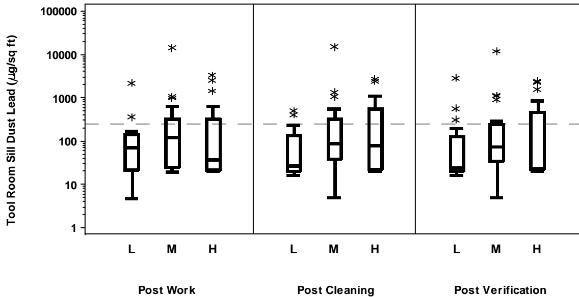
Figure D2.1b. Box Plots of Sill Dust Lead Loading in the Tool Room by Stage and Job Intensity Level
