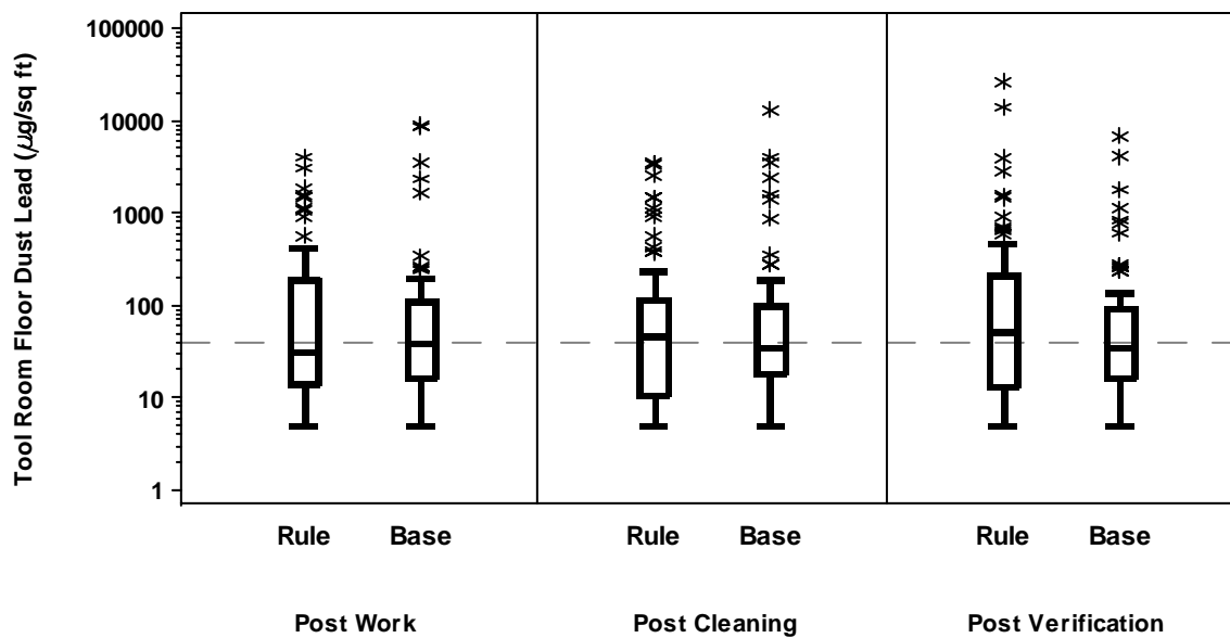
Figure C2.7b. Box Plots of Floor Dust Lead Loading in the Tool Room by Stage and Cleaning Type
