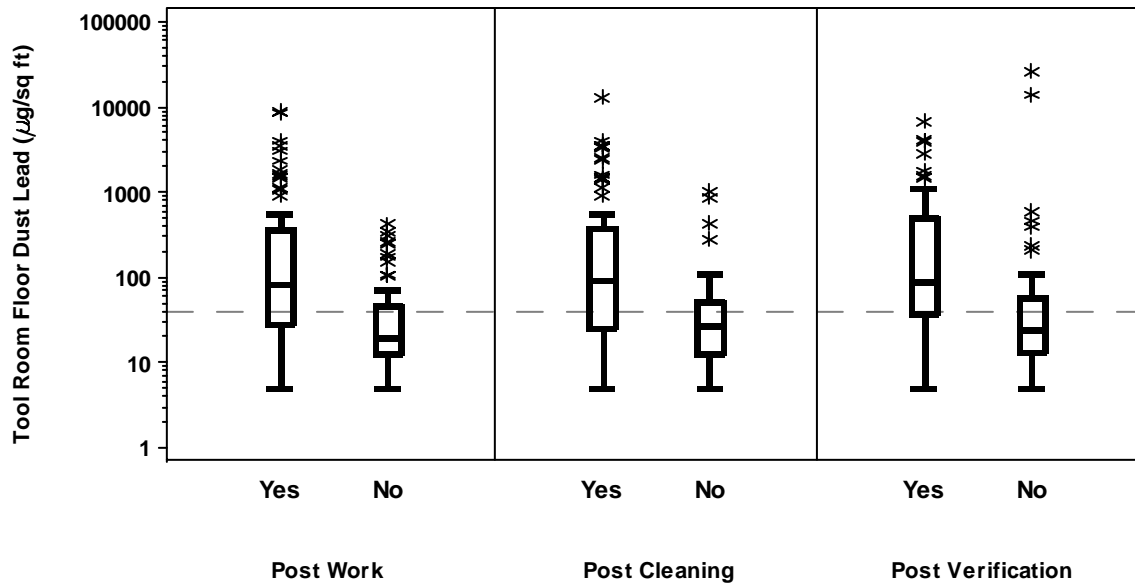
Figure C2.9b. Box Plots of Floor Dust Lead Loading in the Tool Room by Stage and Restricted Job
