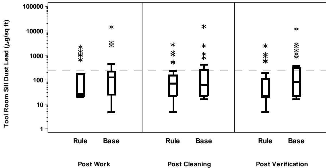
Figure D2.7b. Box Plots of Sill Dust Lead Loading in the Tool Room by Stage and Cleaning Type
