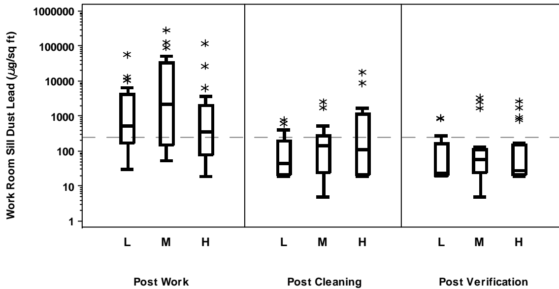
Figure D2.1a. Box Plots of Sill Dust Lead Loading Measured in the Work Room by Stage and Job Intensity Level
