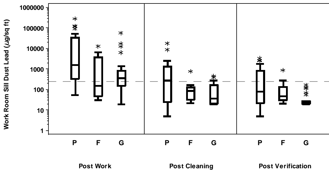
Figure D2.11a. Box Plots of Sill Dust Lead Loading in the Work Room by Stage and Work Room Floor Condition
