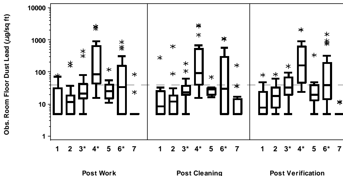
Figure C2.3c. Box Plots of Floor Dust Lead Loading in the Observation Room by Stage and Job Type
