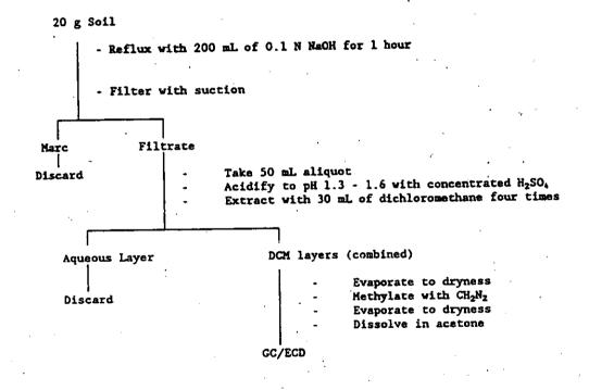
Figure 1. Flow Diagram for BASF Analytical Method Humber A9001 as Applied to Soil.
