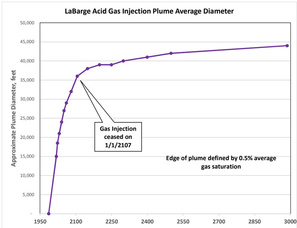
Figure 3.3 – Predicted LaBarge AGI Plume Diameter
