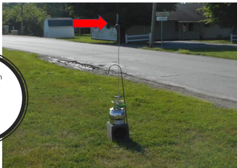
Figure 2 – Outdoor air sampling instrument called a Summa canister.
