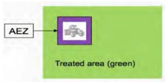
*The AEZ is the purple area around the application equipment. It moves with the application equipment as it proceeds. The AEZ is generally within the treated area, except when the application equipment is near the edges of the treated area.*
