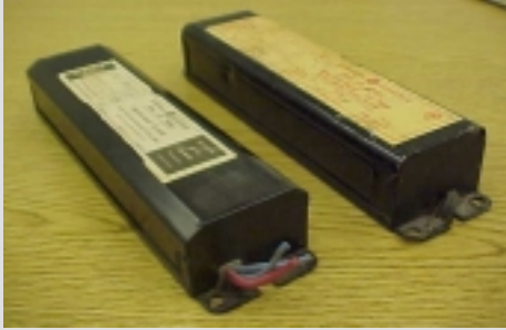
Flourescent light ballasts
