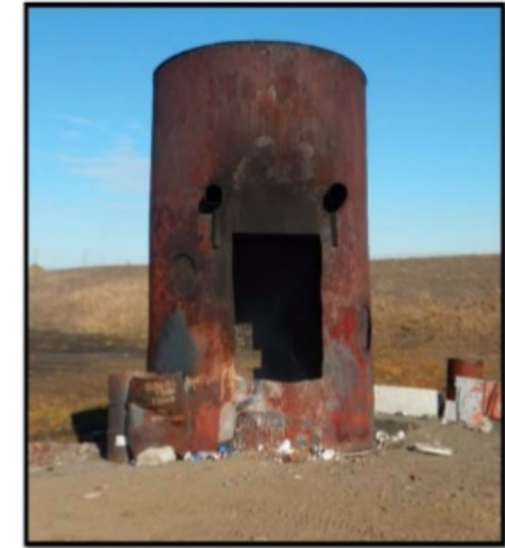
Burn Box constructed from an Old Fuel Tank
