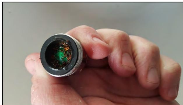
Picture of an aerator with particulate
