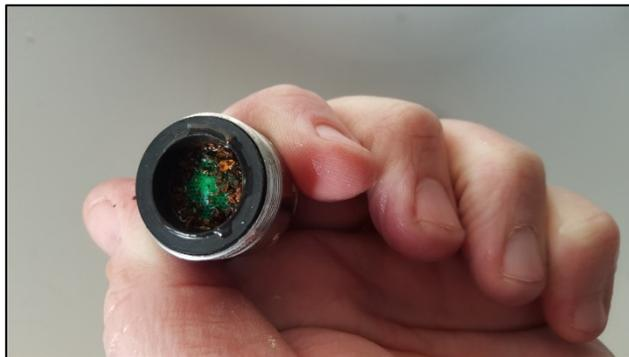
Picture of an aerator with particulate
