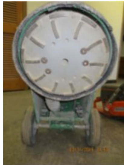
Underside of grinder showing asbestos-containing material from grinding floors.
