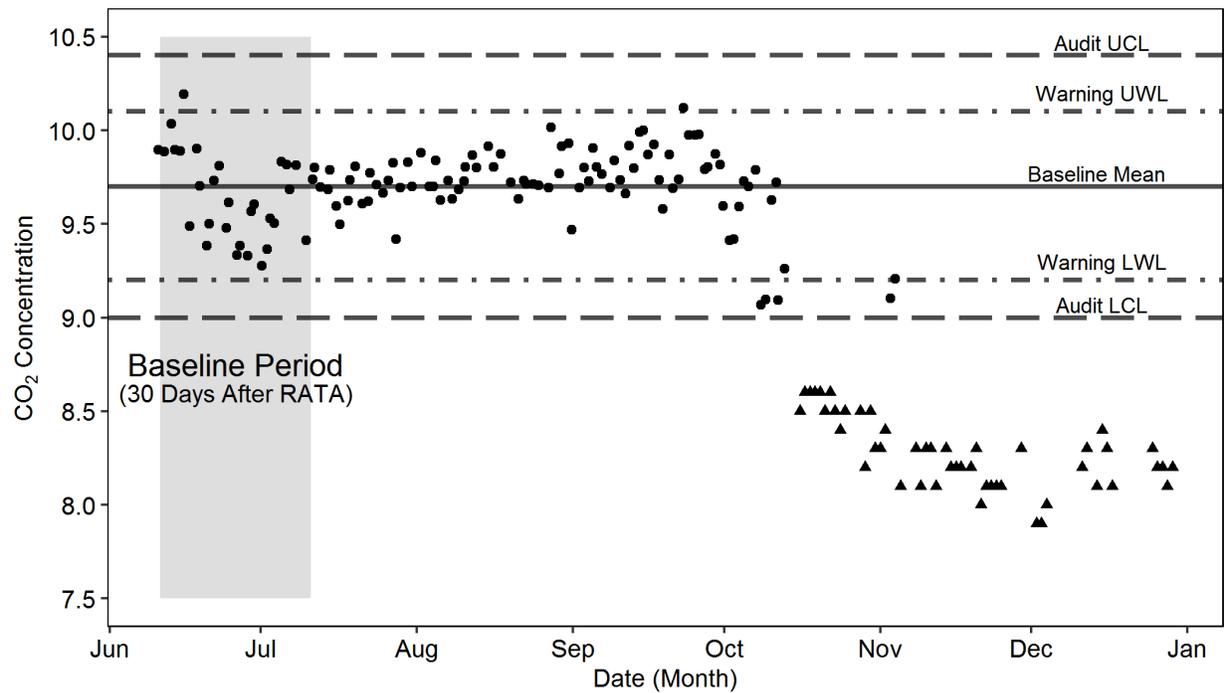
**Figure 4.** Typical CO<sub>2</sub> control chart
