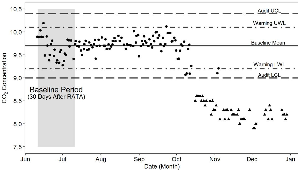
Figure 4. Typical CO<sub>2</sub> control chart
