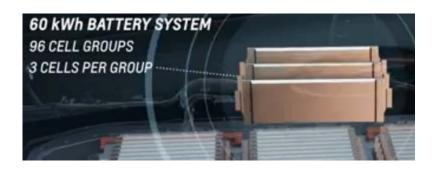
Trend toward flat, floor mounted packs using large, low-profile cells
