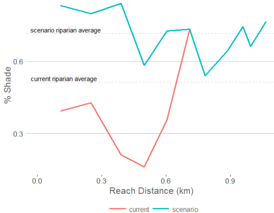
Figure 15 Comparison of average percent shade by reach for current conditions and TMDL scenario. Dotted lines represent average percent shade over the modeled reach.
