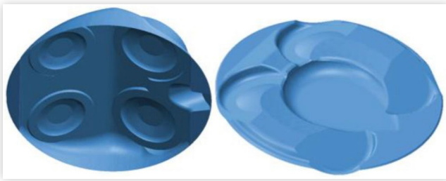
FIGURE 3 10:5:1 combustion chamber surface geometry.
