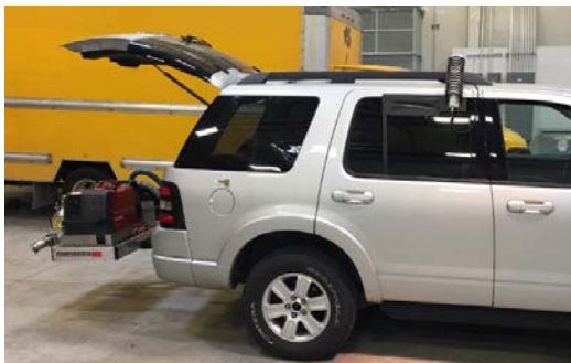
Vehicle equipped with Portable Emissions Monitoring System to measure on-road vehicle exhaust emissions. (EPA OIG photo)
