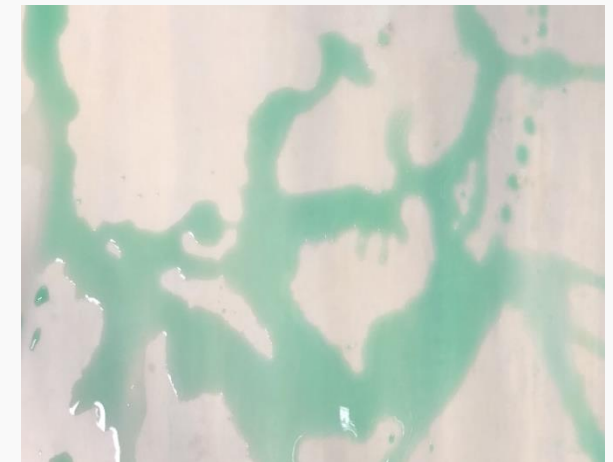
Lack of beading (coalescence) on Latex
