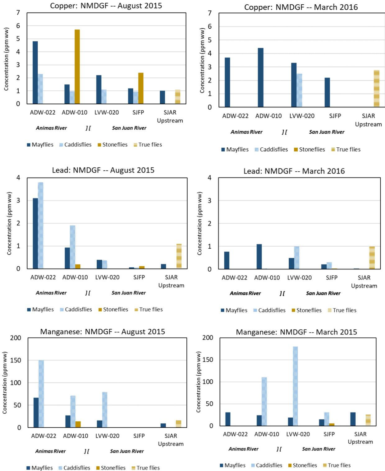
Figure 7.6 Concentration of copper, lead, and manganese measured in benthic macroinvertebrate tissue samples collected by the NMDGF in the lower Animas and upper San Juan rivers in August 2015 and March 2016. The August 2015 samples were collected after the GKM release when deposits were present (see Section 2.3.2, Figure 2.11).
