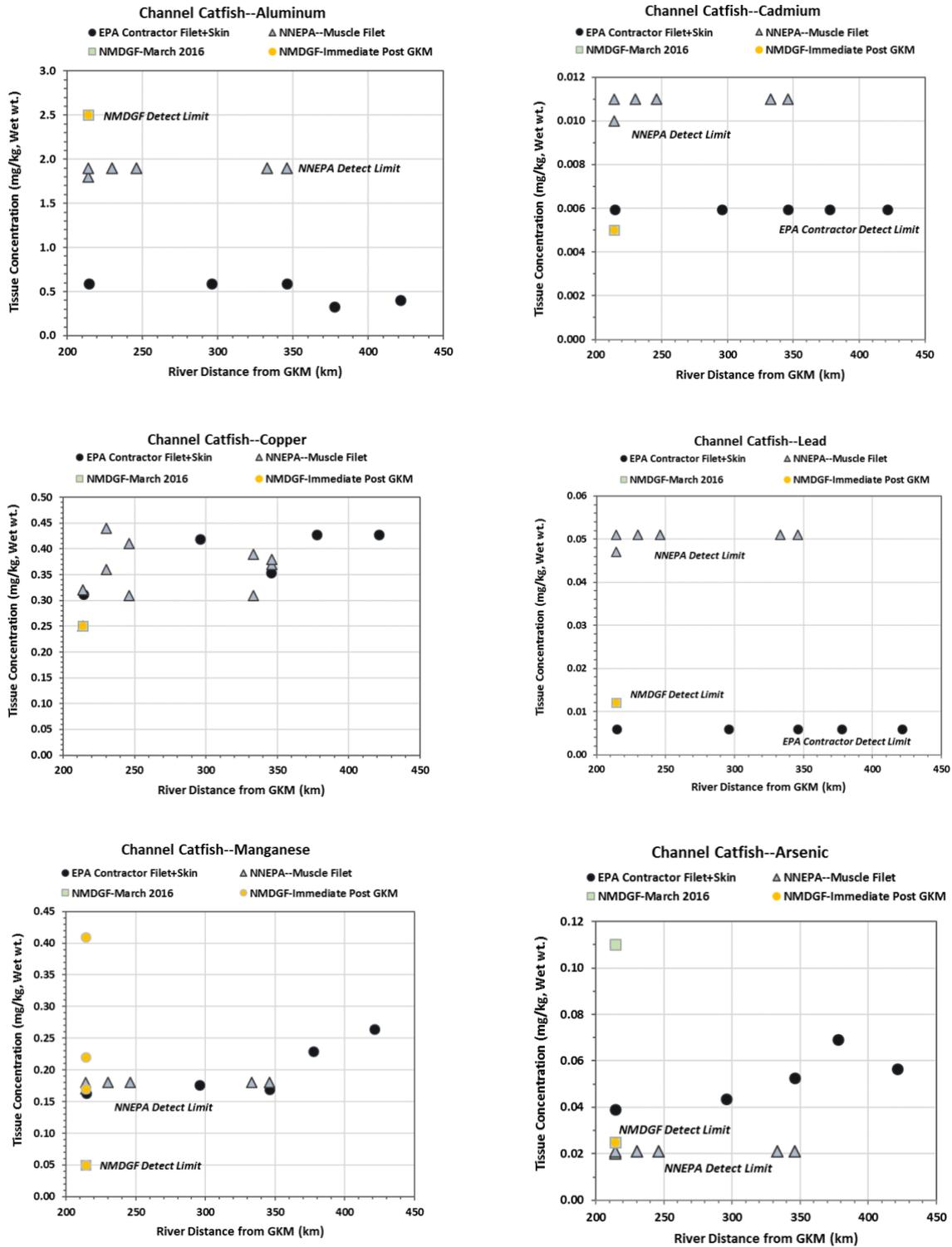
Figure 8.11. Tissue concentration of aluminum and trace metals in channel catfish at multiple locations in the San Juan River. Data were collected by NNEPA and EPA contractors after 2016 snowmelt had returned conditions to background. NMDGF data were collected in August 2015 immediately after the GKM release and in March 2016. DL indicates samples were below the laboratory detection limit, which are shown as 50% reported detection limit.
