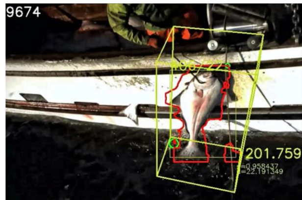
Machine vision view of catch. (Image courtesy of NOAA)
