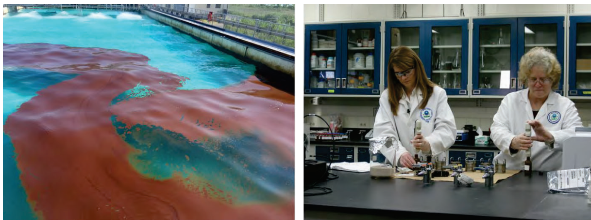
Figure 8: Photo of spill simulations using the Ohmsett wave tank facility at the Naval Weapons Station Earle in NJ (left panel) and laboratory evaluation of the performance of spill-treating agents (right panel).
