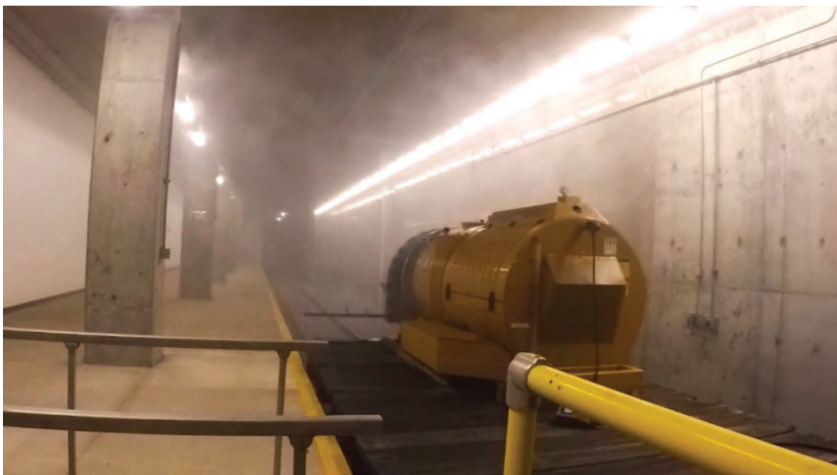
Figure 6: Demonstration of the use of an orchard air blast sprayer for the decontamination of a subway station during an operational technology demonstration
