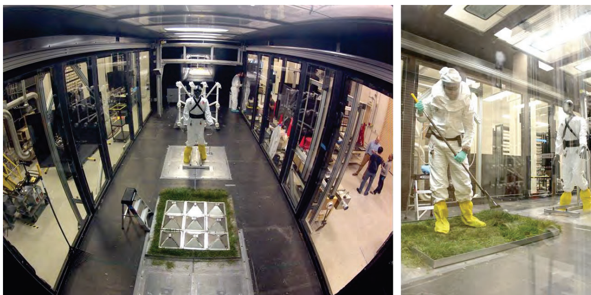
Figure 5: Assessment of reaerosolization of B. anthracis surrogate spores due to typical and response-related human activity (Aerosol Wind Tunnel at EPA's Facility in Research Triangle Park, NC)
