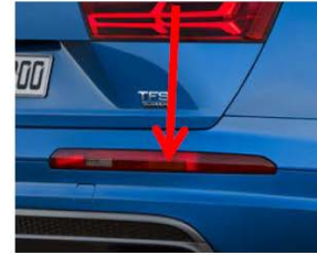
Q Model rear bumper lighting: Tail and turn signal rear and sidemarker
