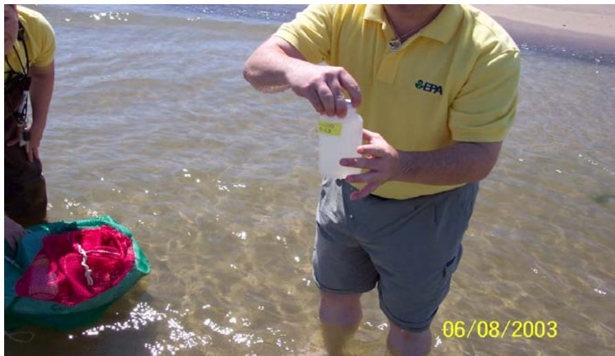
Figure 15. Tightly recapping bottle
