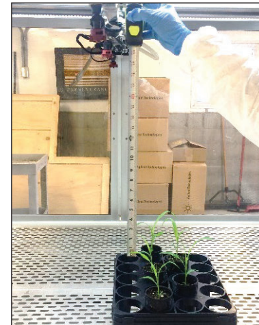
Nozzles spaced 50 cm apart and at 50 cm above the plants.
