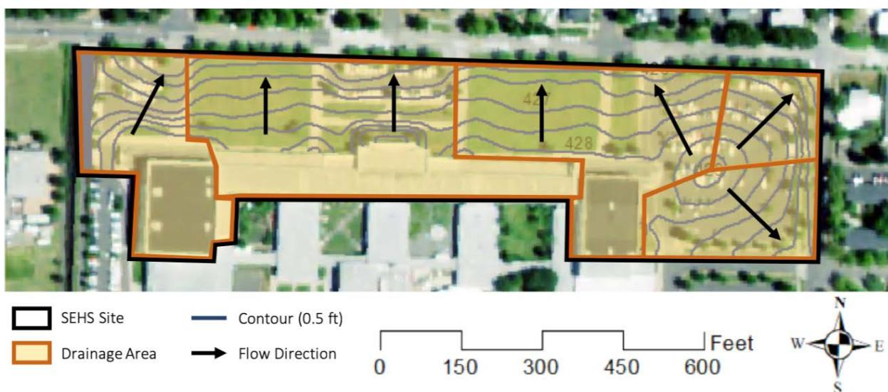
Figure 6: Map depicting demonstration site elevation contours, flow direction, and drainage areas
