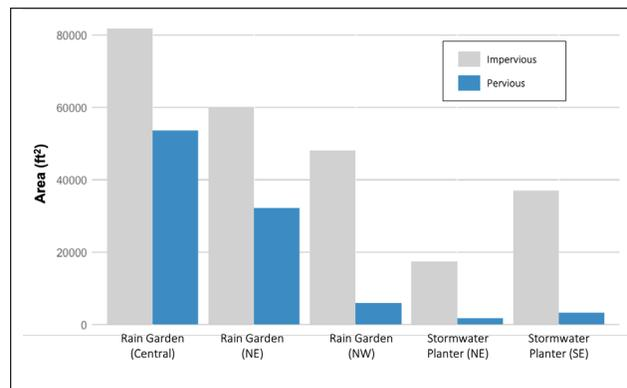
*Figure 7: Pervious and impervious surface area for the five distinct drainage areas*
