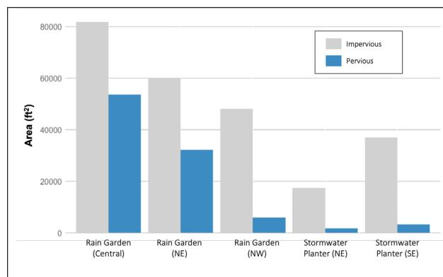
**Figure 7:** Pervious and impervious surface area for the five distinct drainage areas
