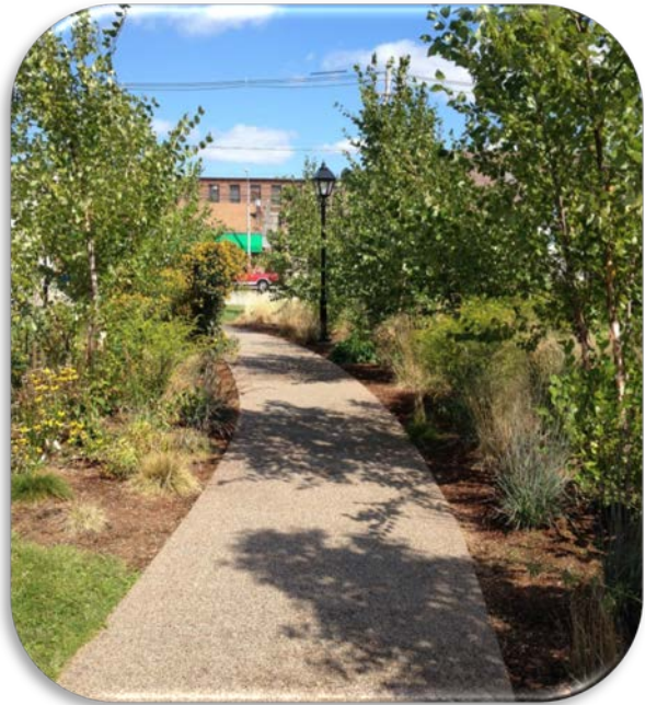
Permeable paving surface made from recycled glass, installed in a new public park in Peabody, Massachusetts.
