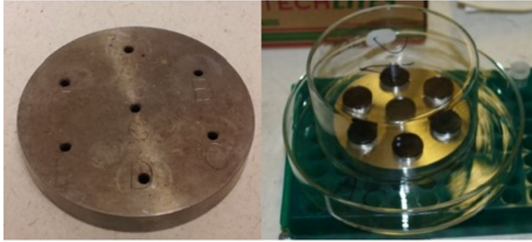
Figure 3-4. Stainless-Steel Stage for Coupon Sterilization
