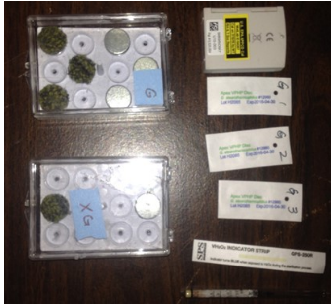
Figure 3-3. Typical Sampling Set with Coupons in Plastic Holders, Temperature and RH Monitor, Three BI discs in Tyvek Envelopes, HP Test Strip, and Dräger Tube
