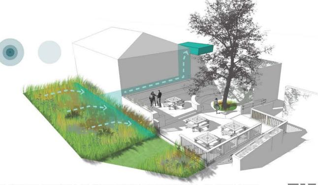
THE CURRENT CHILLER SYSTEM ON CAMPUS WILL BE MOVED TO THE ROOFS OF EXISTING AND NEW BUILDINGS. THE STORMWATER COLLECTION FROM PERIMETER INTERVENTIONS WOULD OFFSET THE WATER USAGE OF THESE SYSTEMS.
