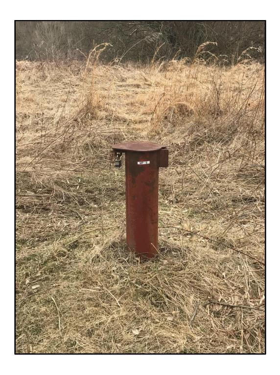
Picture 2: Monitoring Well MW-2D
