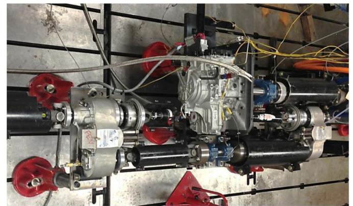
Figure 5. GM6T40 Transmission during testing
