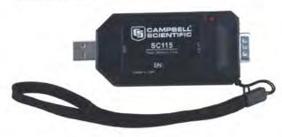
The SC115 is a light-weight, portable instrument that fits in a pocket allowing easy transport between the datalogger and PC.
