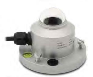
The LP02 includes a bubble level, three adjusting screws, and a cable gland. The bubble level and adjusting screws allow the sensor to be leveled without the use of a leveling base. The gland allows the user to change cables.
