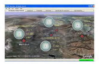
RTMC, a program for displaying the datalogger's data, is bundled with LoggerNet and RTDAQ. Customers may also purchase the RTMCRT and RTMC Web Server clients, which use forms created in the developer mode of RTMC.
