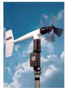
Wind speed is sensed by a lightweight, carbon fiber thermoplastic (CFT), helicoid propeller. Propeller rotation produces an AC sine wave voltage signal with frequency directly proportional to wind speed. Slip rings and brushes are not used.
