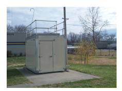
The monitoring site is a stationary equipment shelter located on the grounds of the Firearms Training Center in Louisville, Kentucky. The sample inlet is 4.5 meters above ground level and 52 meters from the nearest road. Upon inspection, the sample lines and monitors were found to be in good condition. The air monitoring site meets the criteria established by 40 CFR Part 58, Appendices C, D, E and G.
