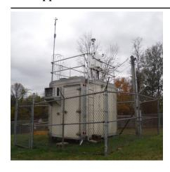
The monitoring site is a stationary equipment shelter located on the grounds of the health department building in Ashland, Kentucky. The sample inlets are 70 meters from the nearest road. Upon inspection, the sample lines and monitors were found to be in good condition.
