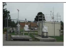
The monitoring site is a stationary equipment shelter located on the grounds of the Fayette County Health Department building in Lexington, Kentucky. The sample inlets are 122 meters from the nearest road. Upon inspection, the sample lines and monitors were found to be in good condition. The site meets the requirements of 40 CFR 58, Appendices A, C, D, E and G.
