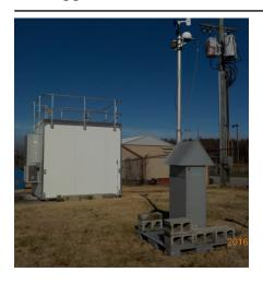
The monitoring site is a stationary equipment shelter located on the grounds of the Livingston County Road Dept. facility in Smithland, Kentucky. The sample inlets are 139 meters from the nearest road. Upon inspection, the sample lines and monitors were found to be in good condition. The site meets the requirements of 40 CFR 58, Appendices C, D, E and G.
