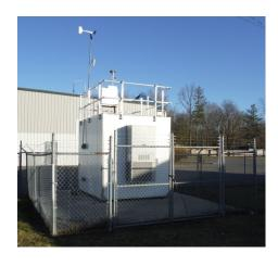
The monitoring site is a stationary equipment shelter located on the grounds of the Middlesboro Airport in Middlesboro, Kentucky. The sample inlets are 92 meters from the nearest road. Upon inspection the sample lines and monitors were found to be in good condition. The site meets the requirements of 40 CFR 58, Appendices C, D, E and G.
