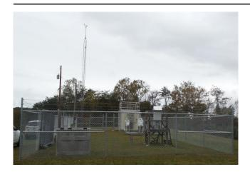
The monitoring site is a stationary equipment shelter in a fenced area located in a remote section of Camp Webb in Grayson, Kentucky. The nearest road is a service road to the site and is 98 meters from the site. Upon inspection, the sample lines and monitors were found to be in good condition. The site meets the requirements of 40 CFR 58, Appendices A, C, D, and E.
