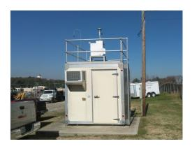
The monitoring site is a stationary equipment shelter located on the grounds of the Somerset Gas Company Warehouse on Clifty Street in Somerset, KY. The sample inlets are 10 meters from the nearest road, which is a dead-end street with little traffic. Upon inspection the sample line and monitors were found to be in good condition. The site meets the requirements of 40 CFR 58, Appendices C, D, and E.
