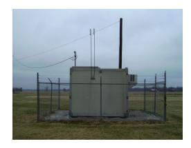
The monitoring site is a stationary equipment shelter located on the athletic fields of the former Lewisport Consolidated Elementary School in Lewisport, Kentucky. The sample inlet is 57 meters from the nearest road. Upon inspection, the sample line and monitor were found to be in good condition. The site meets the requirements of 40 CFR 58, Appendices C, D, E and G.
