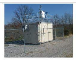
The monitoring site is a stationary equipment shelter located on farmland owned by Northern Kentucky University in Highland Heights, Kentucky. The sample inlets are 23 meters from the nearest road, which is a gravel service-drive for a radio tower. Upon inspection, the sample lines and monitors were found to be in good condition. The site meets the requirements of 40 CFR 58, Appendices A, C, D, E and G.
