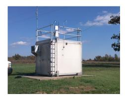
The monitoring site is a stationary equipment shelter located at the residence of 763 Bloodworth Road in Livingston County, Kentucky. The sample inlets are 8 meters from the nearest road, which is an access road for a residence. Upon inspection, the inlet and sampler were found to be in good condition.
