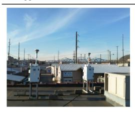
The monitoring site is located on the west end of the roof of the Valvoline Oil complex building in Ashland, Kentucky. The building is one story tall. The sample inlets are 71.3 meters from the nearest road. Upon inspection, the sample inlets and monitors were found to be in good condition. The site meets the requirements of 40 CFR 58, Appendices A, C, D and E.
