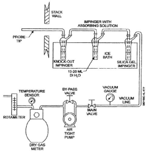
Figure 323-1. Chilled Impinger Train Sampling System
