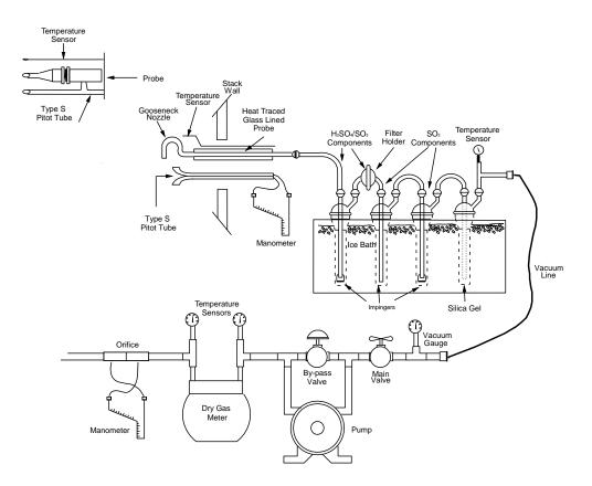
Figure 8-1. Sulfuric Acid Sampling Train
