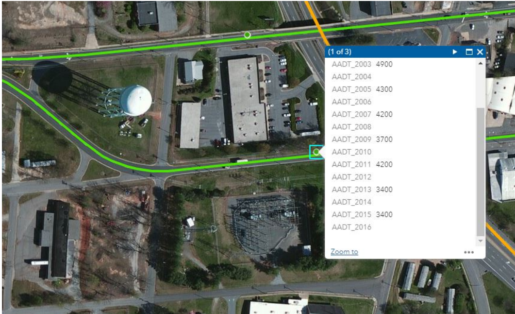
2015 Annual Average Daily Traffic, AADT, for 2 nd Avenue SW, the Hickory monitoring station is located by the water tower AADT obtained from the North Carolina Department of Transportation Traffic Survey Unit
