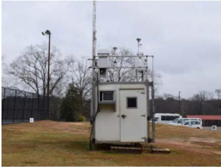
The Irmo site is located in Lexington County near the Town of Irmo. This site has a sampler for PM<sub>2.5</sub> and continuous monitors for SO<sub>2</sub>, BC, and PM<sub>2.5</sub>. Additionally, this site has samplers collecting Carbonyl and SVOC samples on a 1:6 schedule. The sample inlets are 39 meters from the nearest road.
