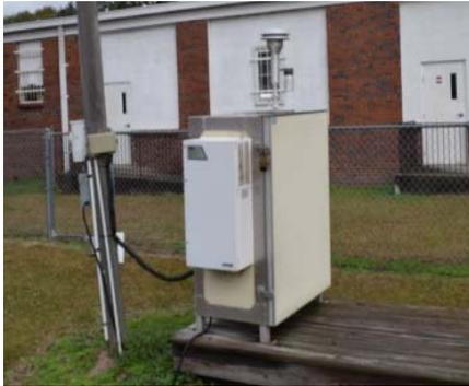
The Howard High #3 site is located in Georgetown County on the grounds of Howard High School and supports a PM<sub>10</sub> monitor. PM<sub>10</sub> monitoring in this area of Georgetown has been ongoing since 1970, when the original Howard High site was established. The sample inlet is 49.7 meters from the nearest road.
