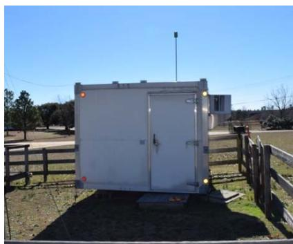
The Sandhill Experimental Station site is located in northeastern Richland County, downwind from the Columbia metropolitan area. This site is located in a rapidly urbanizing portion of the city of Columbia. The Sandhill site measures Ozone and NO<sub>2</sub>. The sample inlets are 31 meters from the nearest road.
