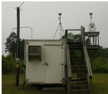
The Trenton site is located in southeastern Edgefield County. Trenton was originally established to monitor for Ozone crossing into South Carolina from Georgia. The Trenton site monitors for Ozone, intermittent PM<sub>2.5</sub>, and continuous PM<sub>2.5</sub>. The sample inlets are 30 meters from the nearest road.
