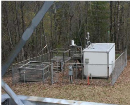
The Long Creek site is located on Round Mountain in northwest Oconee County. The Long Creek site was also established as part of the Southern Oxidant Study. It provides a unique vantage point for monitoring the impacts of transported pollutants. Long Creek has continuous monitors for Ozone, SO<sub>2</sub>, and PM<sub>2.5</sub>. The sample inlets are 30 meters from the nearest road.
