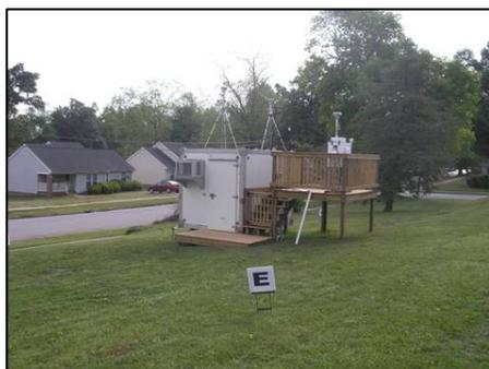
The Greenville ESC site is located in the city of Greenville and was established on April 11, 2008. This site supports a PM<sub>2.5</sub> sampler and continuous monitoring for PM<sub>2.5</sub>. It also supports PM<sub>10</sub>, SO<sub>2</sub>, NO<sub>2</sub>, Sulfate, BC, and measurements for wind speed and wind direction. The sample inlets are 15. meters from the nearest road.
