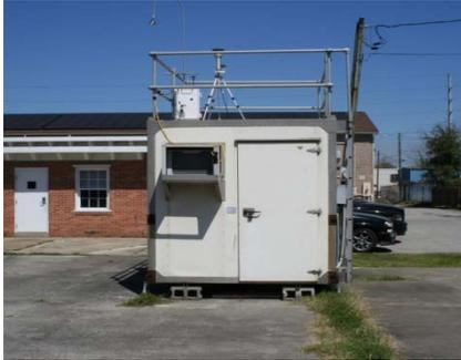
The Jenkins Ave. Fire Station site is located in the city of North Charleston behind a fire station in an urban and central city setting. The Jenkins Ave. Fire Station site supports monitors for PM<sub>10</sub>, SO<sub>2</sub>, and NO<sub>2</sub>. The sample inlets are 33.5 meters from the nearest road.
