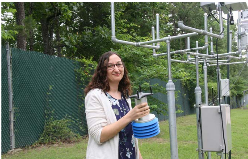
EPA scientist Ingrid George holds an SPod, a fenceline monitoring system developed by EPA that can identify air pollution plumes from leaks or other fugitive emissions at the perimeter of industrial facilities.
