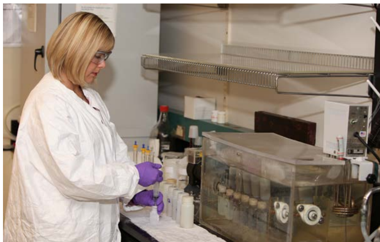
EPA researcher Karen Bradham uses a “virtual stomach” that mimics human digestion to determine if arsenic and lead in contaminated soils are bioavailable.
