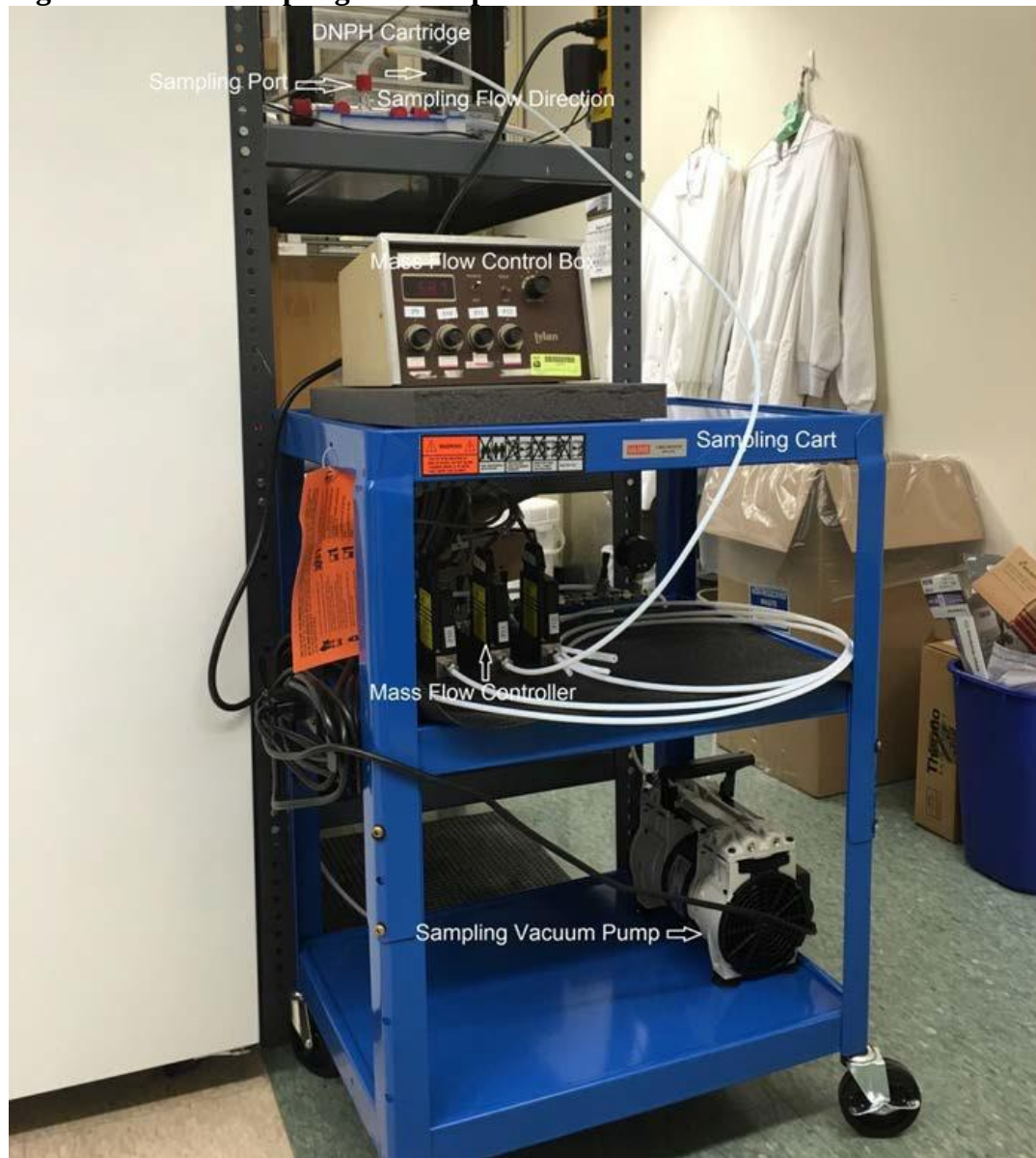
Figure 3. DNPH sampling cart setup
