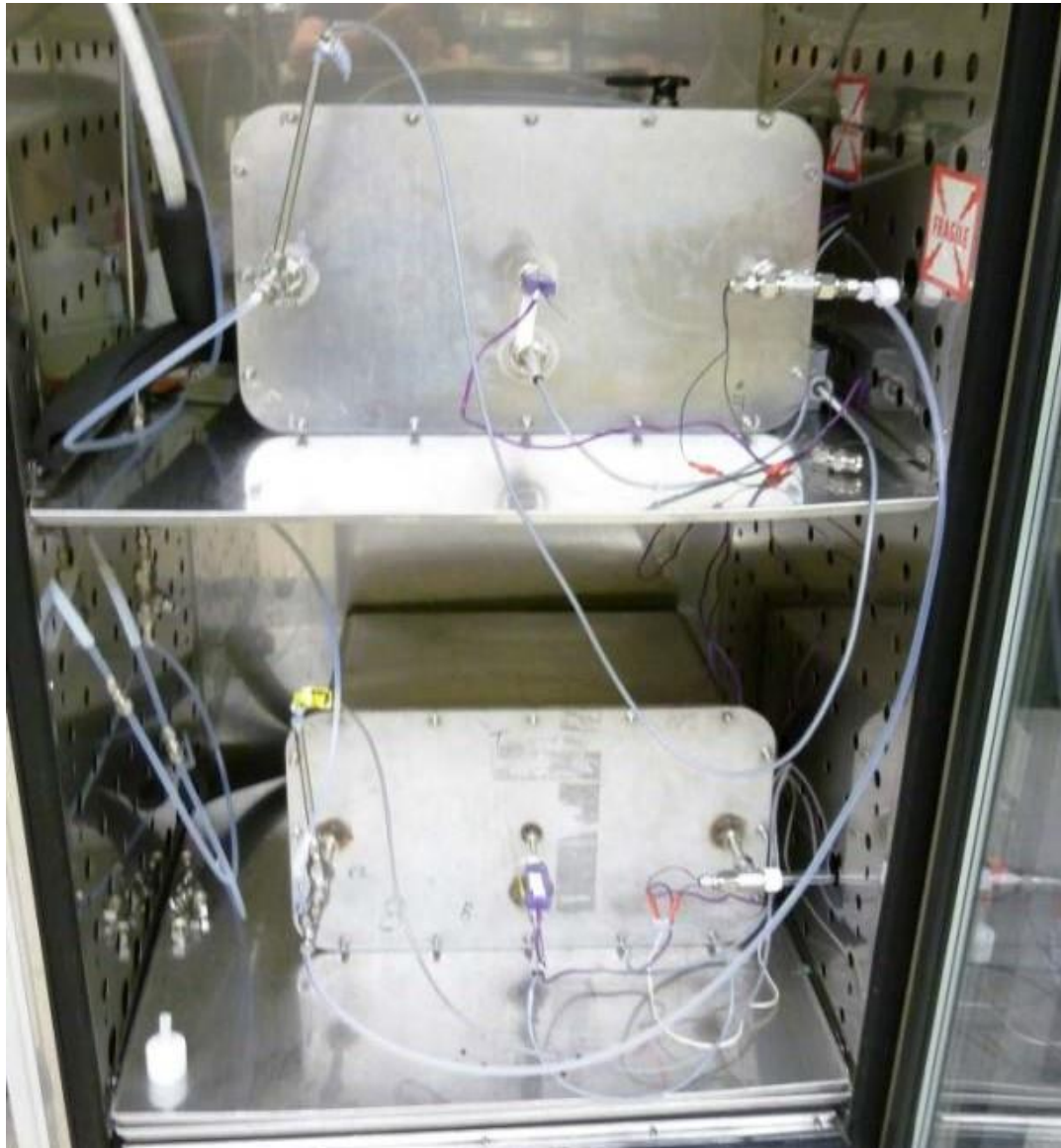
Figure 1. Picture of two small environmental chambers in the Forma Scientific Model 39900 incubator
