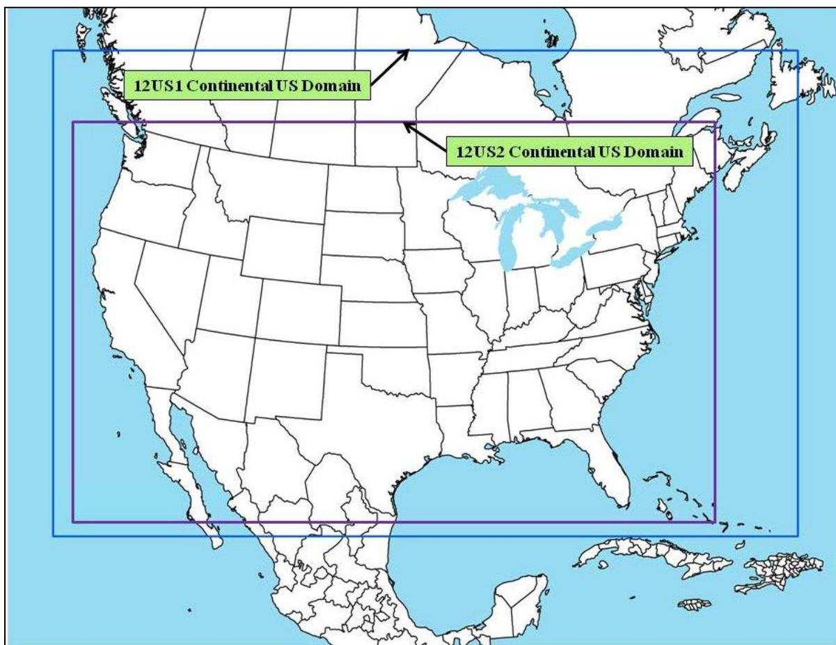
All grids use a Lambert-Conformal projection, with Alpha = 33°, Beta = 45° and Gamma = -97°, with a center of X = -97° and Y = 40°. Table 3-2 describes the grids for the three domains.
