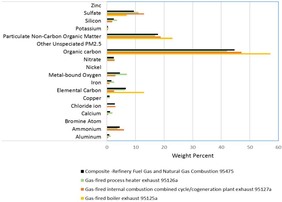
**Figure 3-4. Comparison of PM profiles used for Natural gas combustion related sources**
