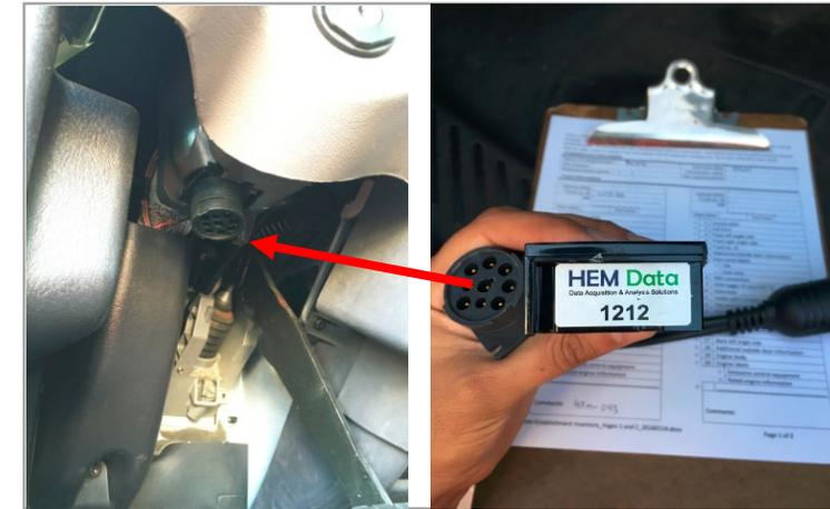
*Mini-logger that fits on the in-cab J1939 connector, to acquire vehicle diagnostic data*
