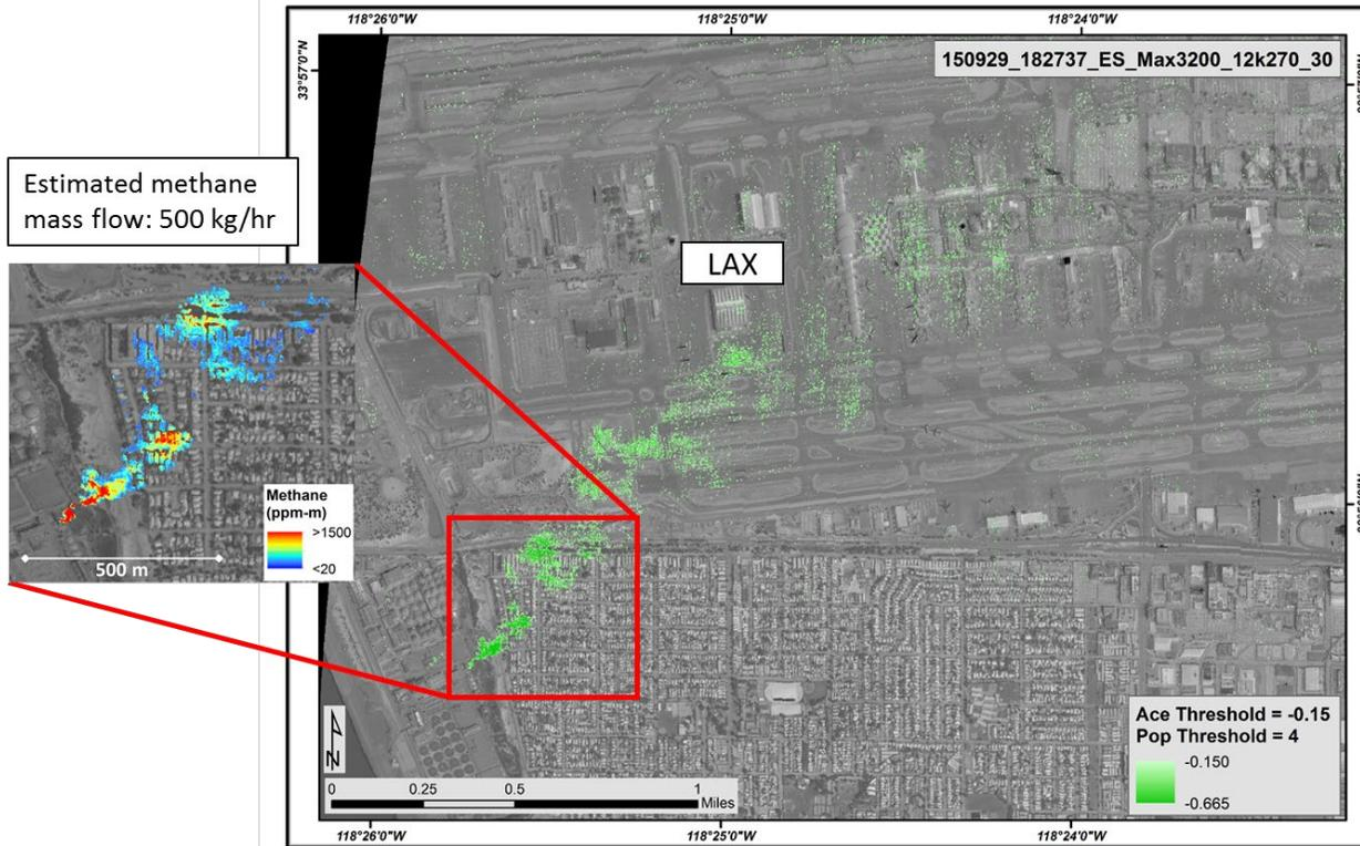
Methane release from wastewater treatment plant; plume length ~4 km
