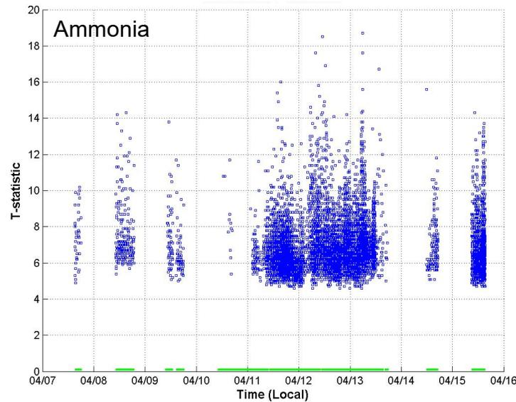
Observations suggest that venting of overpressured HVAC systems is synchronized within a few hours of local noon
