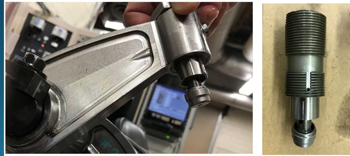
Cylinder-deactivation through Eaton's collapsible lifter
