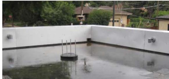
*Photo 29.2 Example of flood test at a Denver residential green roof.*
