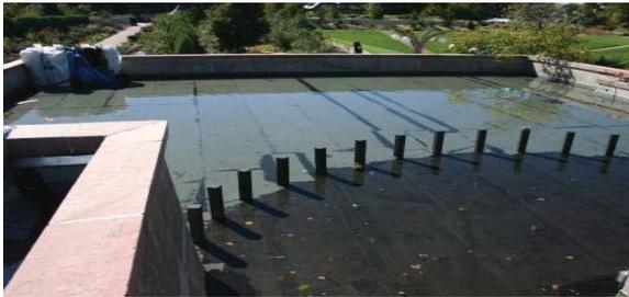
*Photo 29.1 Example of flood test at the Denver Botanic Garden green roof.*
