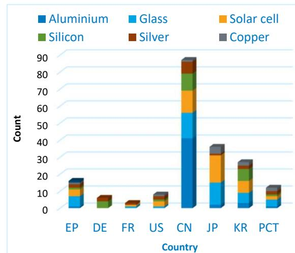
Fig. 2-11 Recovered materials for c-Si PV module recycling patents by country
