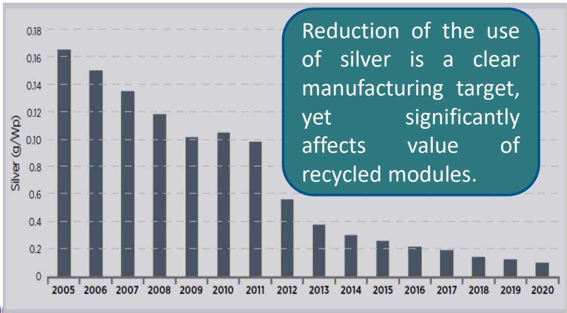
Reduction of the use of silver is a clear manufacturing target, yet significantly affects value of recycled modules.
