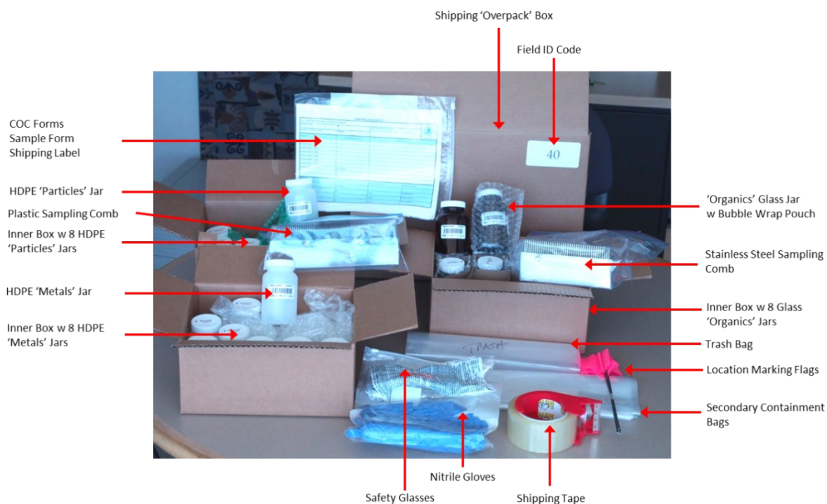
Figure 3-8. Sample collection kit for metal, organic and particle sample collection at synthetic turf fields. [COC = Chain of custody; HDPE = High-density polyethylene]
