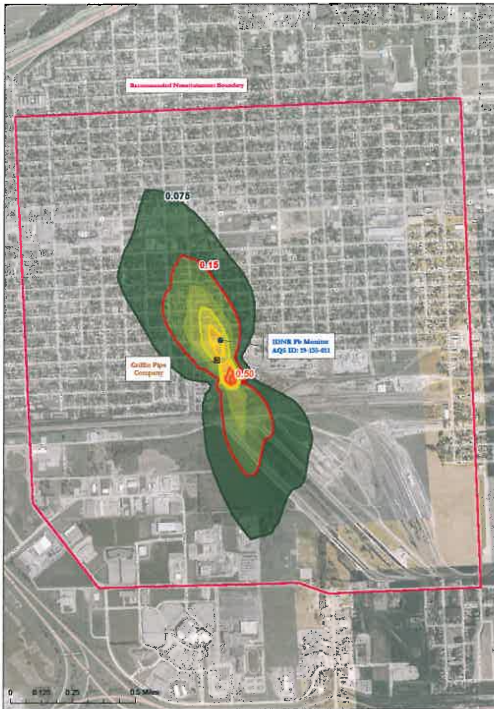
Figure 8. EPA Air Dispersion Model Result – Absent Baghouse Controls
