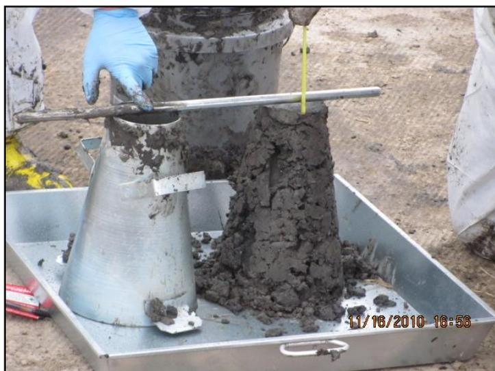
**Photo 4-20. 2-Inch Slump Test of TSCA Material**
