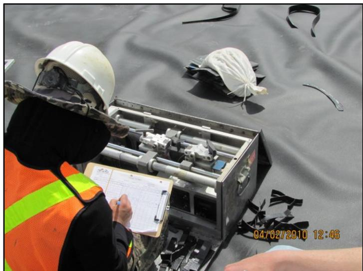
**Photo 3-2. Destructive QC Testing of Geomembrane at Non-TSCA Dewatering Pad**
